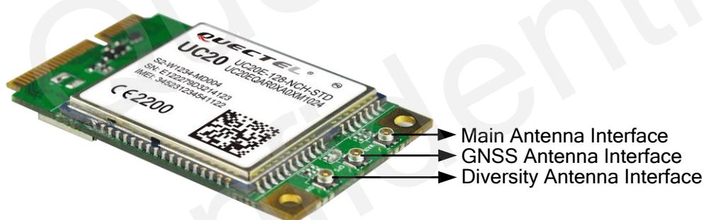
Figure 17: UC20 Mini PCIe Antenna Interface
