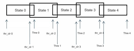
When temperature exceeds the "current state" "threshold", the thermal mitigation algorithm searches the next state that this temperature is lower than its "threshold". After it finds it, the "current state" is updated to that "state" and then it checks whether "action" is "mitigate", if yes, then it activates the mitigation according to the "action info" of the "current state".
