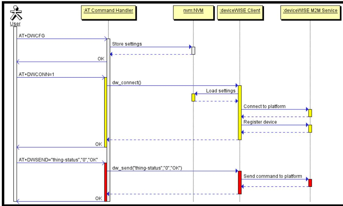
Figure 5: Basic Interaction Diagram of IOT Platform
