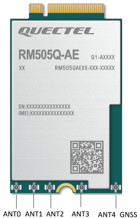
Figure 28: Antenna Connectors on RM505Q-AE
