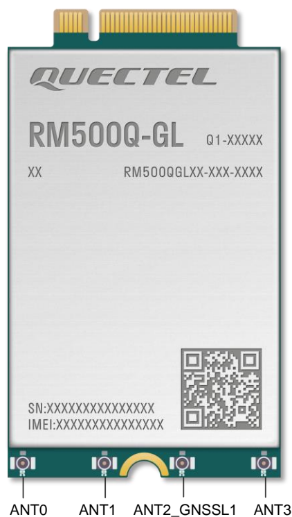
Figure 26: Antenna Connectors on RM500Q-GL
