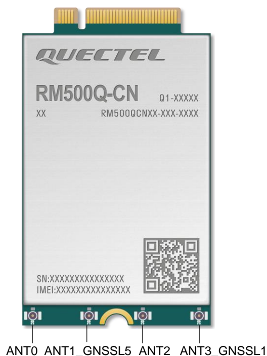
Figure 29: Antenna Connectors on RM500Q-CN
