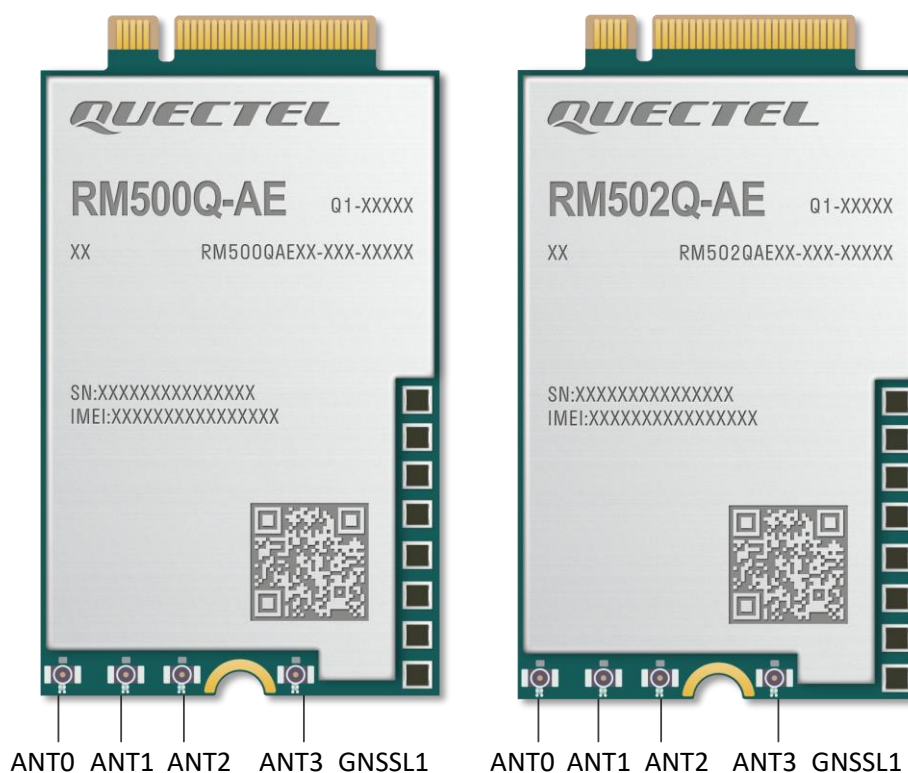
Figure 27: Antenna Connectors on RM500Q-AE & RM502Q-AE
