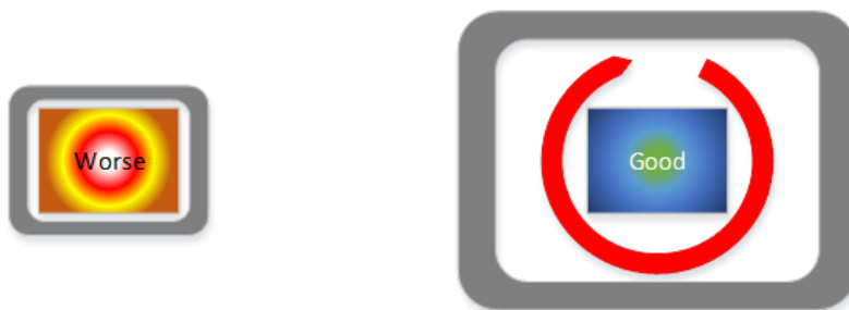
Figure 19: Enlarge Internal Space for Better Air Convection
