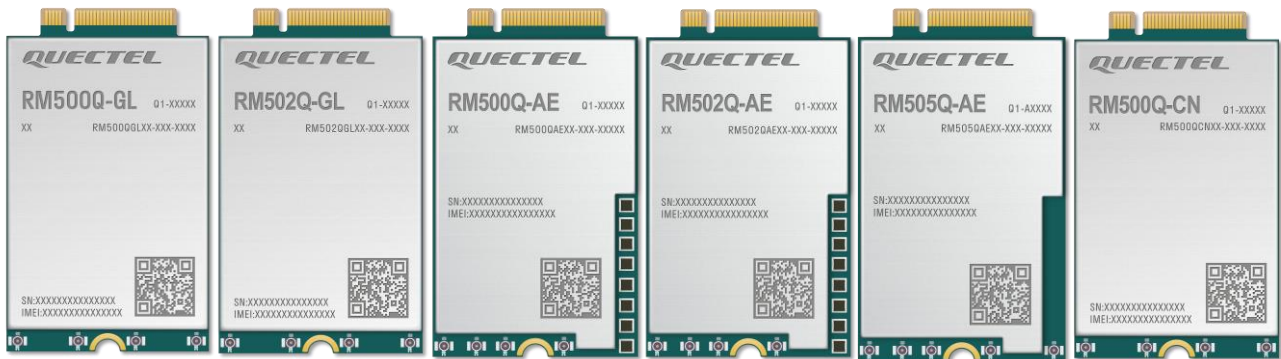
Figure 1: Top Views of RM50xQ Series Modules
