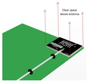
The location within the device should ideally be along any outer edge. The antenna can be in direct contact with any surface.
