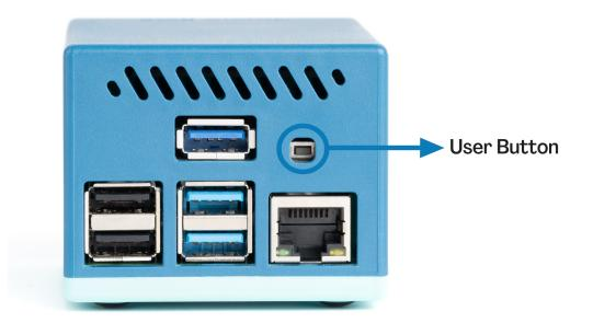
• **User Button:** It is a programmable user button that is connected to GPIO20. It reads HIGH by default.
