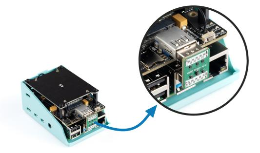
The USB Bridge serves the purpose of connecting the 5G module with the USB 3.0 port of the Raspberry Pi. This design choice was made in favor of using a USB cable, as it provides a robust, aesthetic, and space-saving solution. Rather than a standard straight cable connection, the USB Bridge has been specifically designed with EMI/EMC filtering components to ensure faster and more efficient data transmission.
