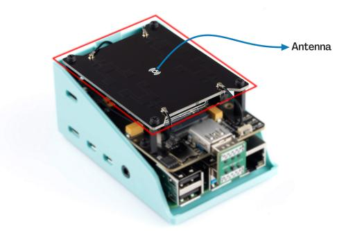
This antenna has been specifically designed and produced by Sixfab engineers, focusing on 5G bands and frequencies, exclusively for the Jumpstart 5G product.
